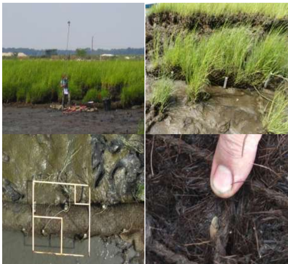
Figure 7. Results after log installation show sediment trapping with algal mats and survival of planted marsh grass and ribbed mussels.
